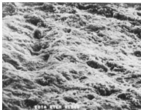
FIGURE 8 HA plate etched with 0.5% EDTA for 2 min (SEM \times 1500 ).
