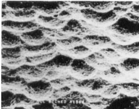
FIGURE 4 HA plate etched with 0.5 HCl for 10 min, washed with methanol (SEM \times 1500 ).
