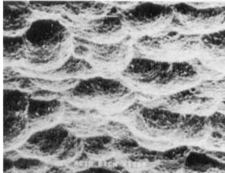
FIGURE 3 HA plate etched with 0.5% HCl for 10 min, washed in water (SEM, \times 1500 ).
