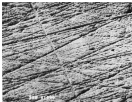
FIGURE 2 Surface of HA plate ground with 600 SiC grit and ultrasonically cleaned with methanol and water (SEM, \times 1000 ).
