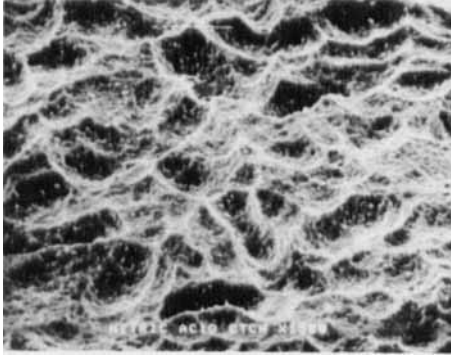
FIGURE 5 HA plate etched with 0.5% HNO 3 for 10 min, washed with methanol (SEM \times 1500 ).
