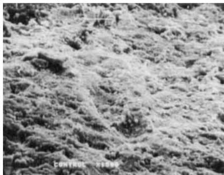
FIGURE 1 Ground surface of as-received HA plate (SEM, \times 1500 ).
